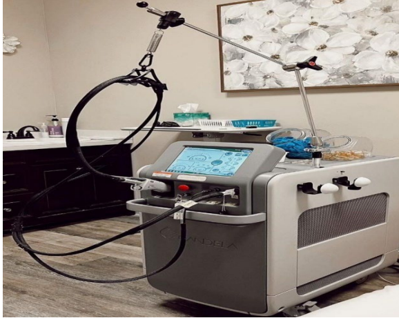
Figure 2: Candela laser hair removal device. Model: Gentle Max Pro, Type: Dual-wavelength medical laser system, Wavelength: 755 nm (Alexandrite) and 1064 nm (Nd:YAG), Pulse duration 0.25–100 ms.
